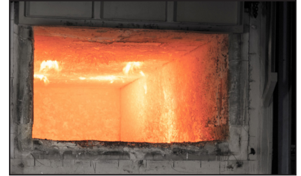
This stack heating device uses heat exhaust to preheat aluminum before it is melted, thereby conserving natural gas.
